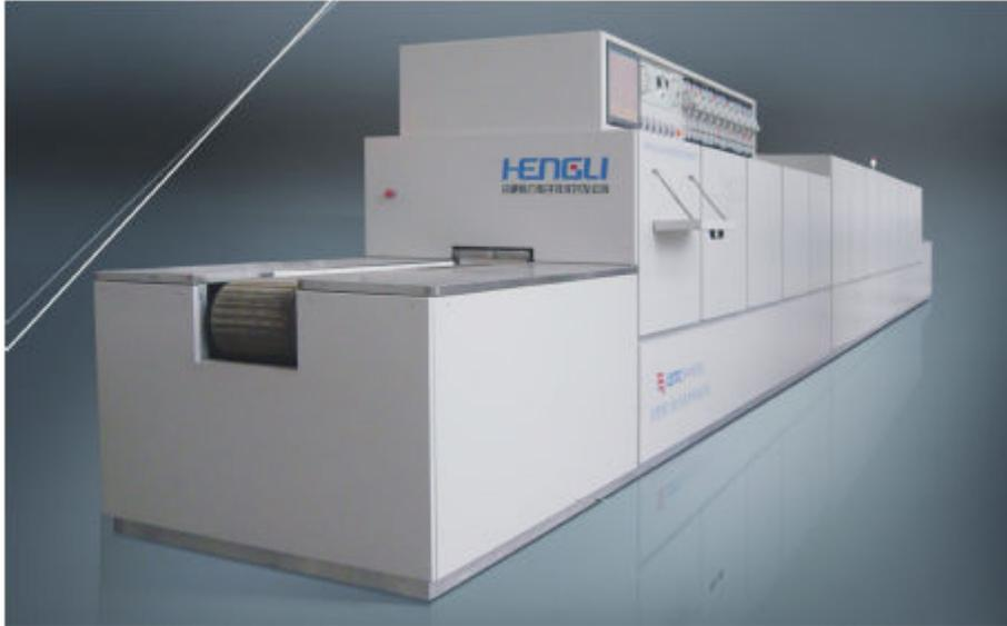
HengLi RSK3003Z-09A furnace is widely used for solar cell contact drying, firing and metallization.
