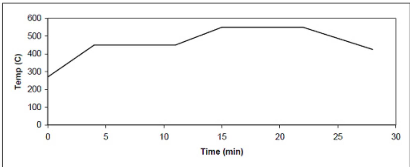
Figure 2: Selenization profile of CIGS solar Cell
