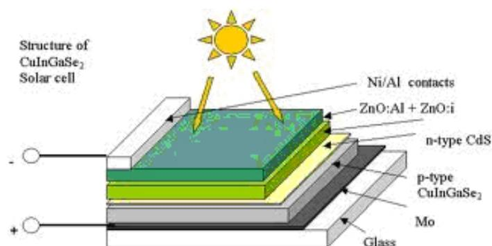
Figure 1: Material Stack up of CIGS solar Cell
